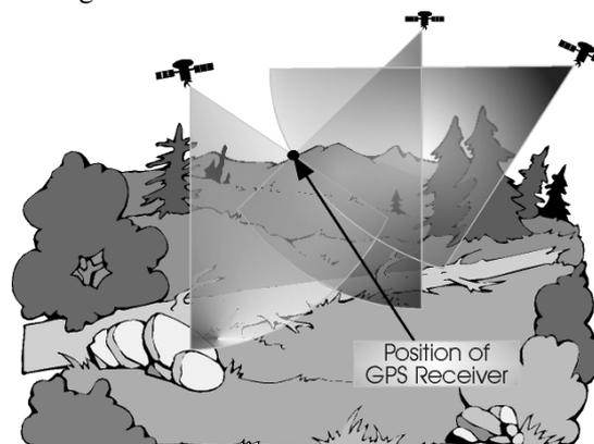
Figure 1. Evaluating position of GPS unit in 3D space as a distance from three satellites.
