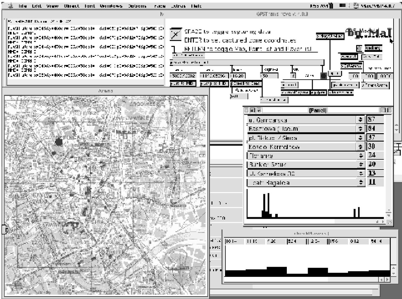
**Figure 3. NMEA Receiver Module written in Max 4.0, which has been used during *GPS Trans 2 & 3*.** Screenshot presents Map Window (purple dot shows current position of car), window with list of Nearest Points, and Players Window, which displays volume of currently played back samples.
