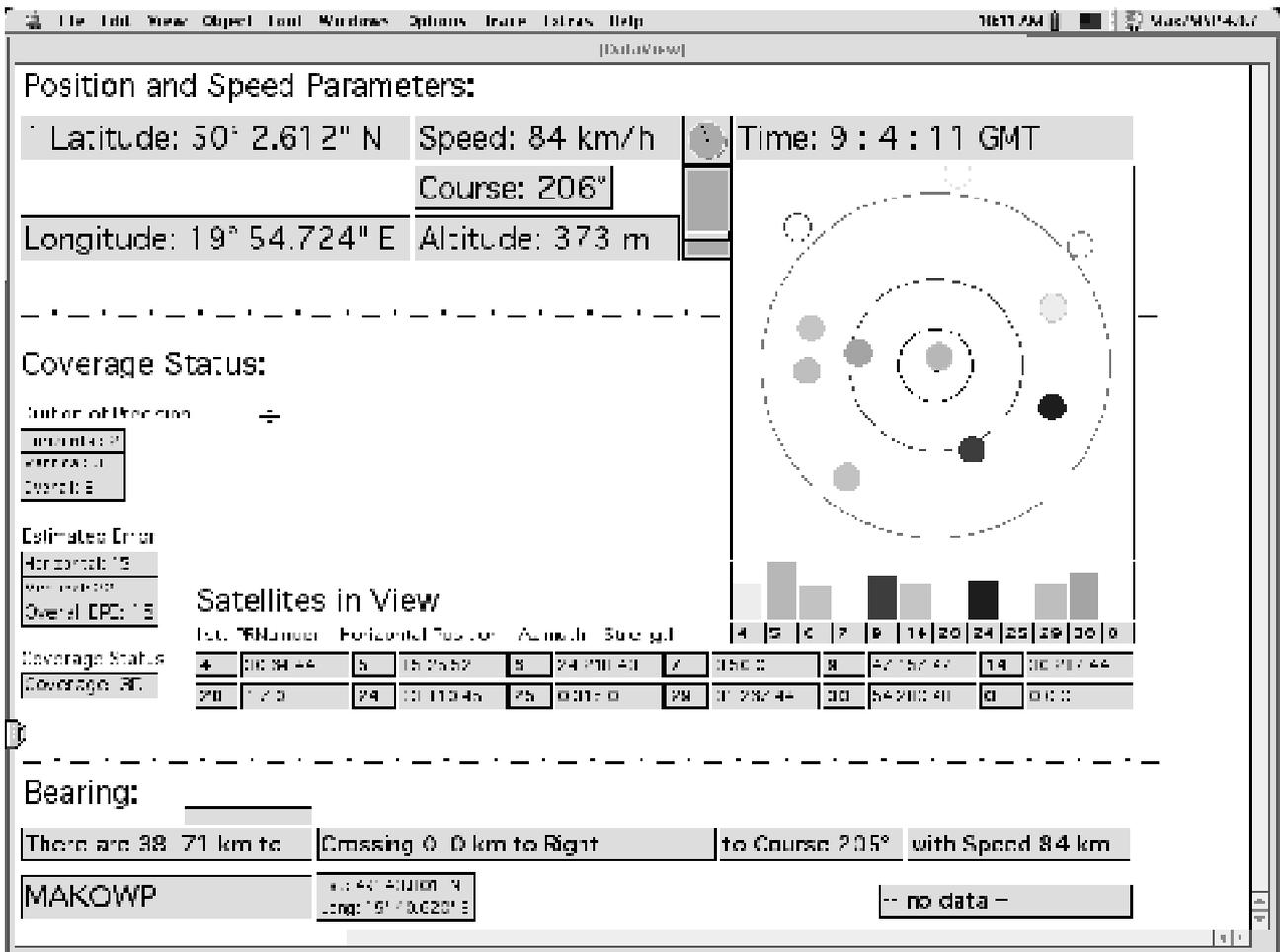
**Figure 5. The Complete NMEA Interface done in Max. On the screen appears all data send by *Garmin GPS 12* unit.**
